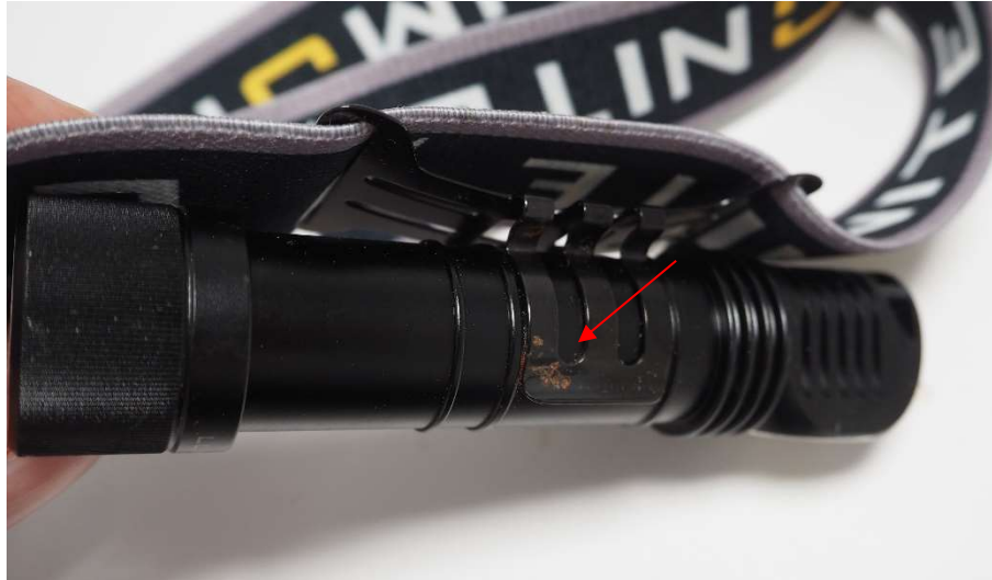
Figure 6. Corrosion marks after test from attachment part.
